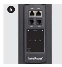
Step 5 - Power on the PDU - Set the PDU level according to Step 1
